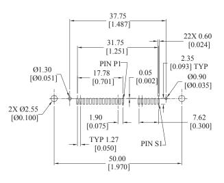
RECOMMENDED PCB LAYOUT TOLERANCE: ± 0.05 [0.002]
