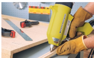
Adhesive bead applies neatly to countertop edging to eliminate nails and the extra work of putty and sanding.
