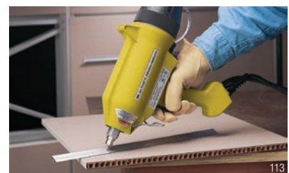
Adhesive bonds extruded aluminum bracket to the laminate covering of a honeycomb panel.
