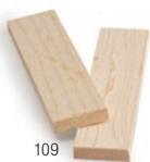
Two pieces of oak are edge spliced with the 3M™ Scotch-Weld™ PUR Adhesive System.
