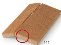
The wood fails before the bond line in this test and many other applications.
