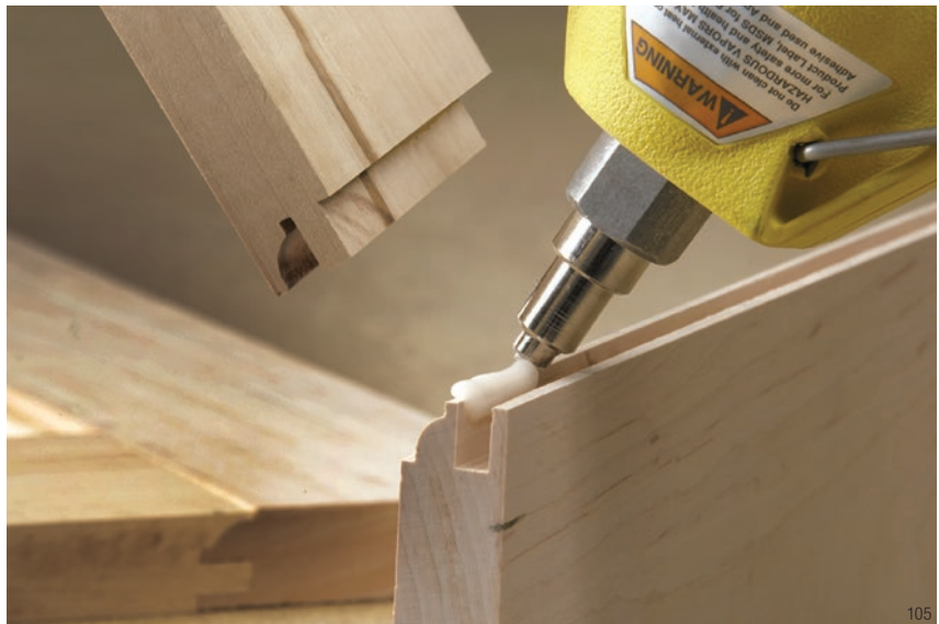
Choice of viscosities and open time to match application requirements for bonding wood to wood as well as wood to other substrates.
