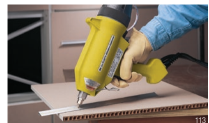
Adhesive bonds extruded aluminum bracket to the laminate covering of a honeycomb panel.
