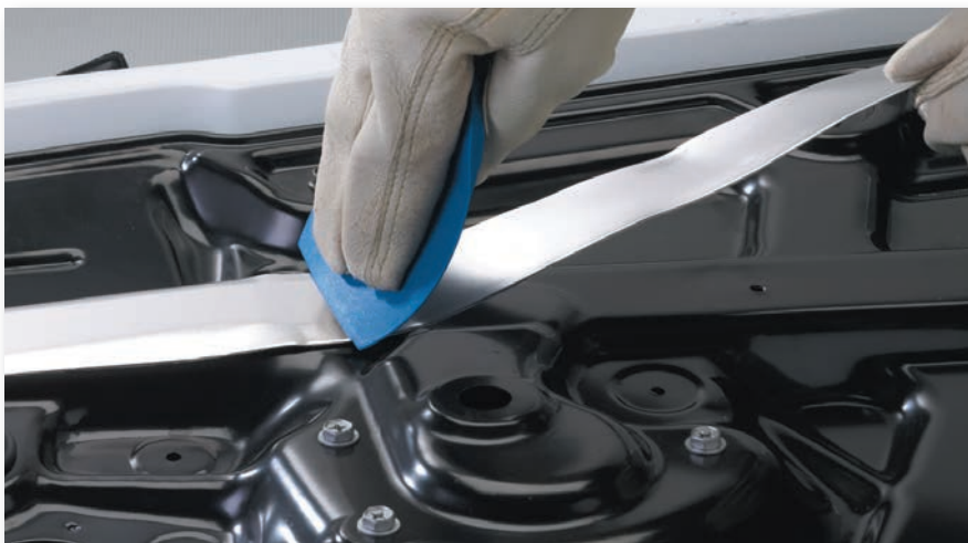
Applied with a 3M™ PA-1 Wiper to the inside of a car door, 3M™ Damping Foil 2552 effectively damps noise and vibration with as little as 10% surface coverage. Optimized acrylic on a dead soft aluminum constraining layer converts vibrational energy to negligible heat that readily dissipates.
