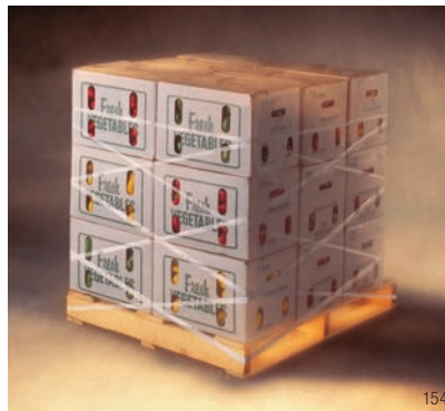
“X”-pattern can contain loads for shipment anywhere.
