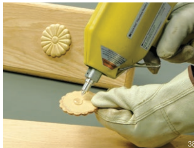
Bond wood or plastic trim to wood cabinet doors.
