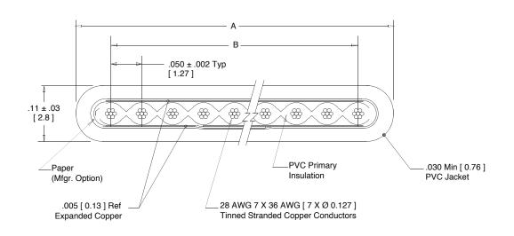
Note: Red marking on edge of primary cable designates wire #1.
