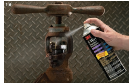
166 Freeing rusted nuts, bolts and frozen threaded parts are only a few of the many applications for 3M™ 5-Way Penetrant.
