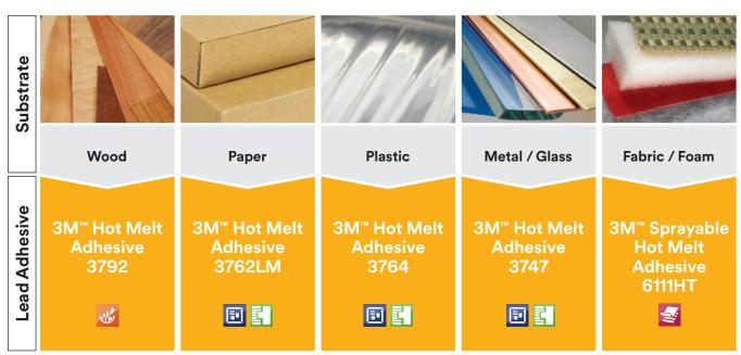
Hot Melt Adhesive is dispensed at 350-385°F. Low Melt Adhesive is dispensed at 250-270°F.
