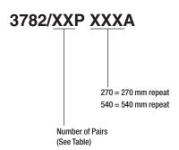
Note: Available in standard 100 ft rolls. Contact 3M for availability of additional conductor counts and/or custom roll lengths.
