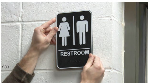
3M™ Double Coated Urethane Foam Tapes bond plastic signs to painted cinder block. The foam fills gaps between irregular surfaces. Various foam thicknesses are available for surface conformance based on the degree of roughness.
