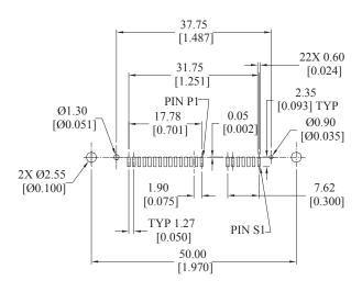
RECOMMENDED PCB LAYOUT TOLERANCE: ± 0.05 [0.002]
