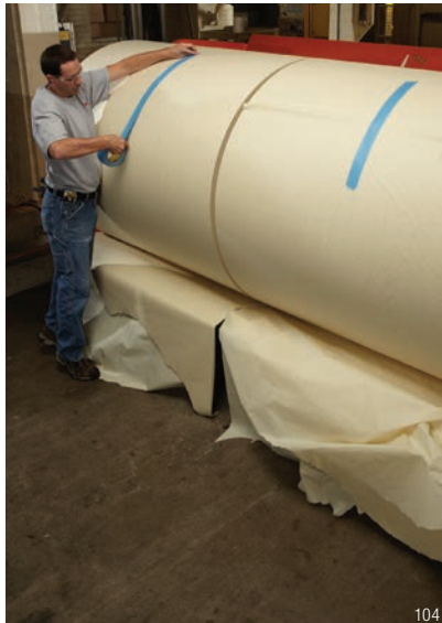
High tack 3M™ Temporary Single Coated Repulpable Tapes are available in white, blue, and kraft for dependable core starting, roll closing and butt splicing.
