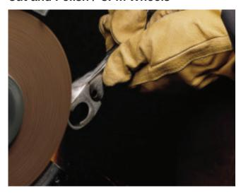
Cut and Polish / CPM Wheels are heavy duty wheels for more aggressive blending and finishing. These long lasting wheels perform well on tough blending and finishing applications such as removing surface defects, coarse grindlines, blending forging marks and machining mismatches while leaving a uniform grain finish.
