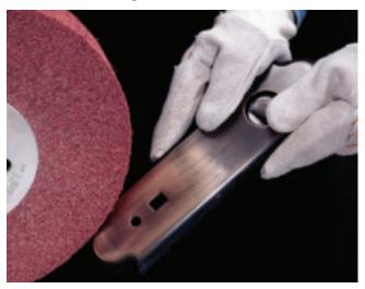
Highly conformable Metal Finishing Wheels are designed to apply uniform and consistent satin/antique finishes. They are used effectively to blend and match #3 or #4 mill finishes on stainless steel and to create brushed or satin finishes on cutlery.
