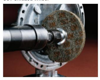
SST Unitized Wheels offer the same deburring and finishing advantages as SST Convolute Wheels (SST Deburring Wheels; refer to page 8). The unitized version of the SST wheel is recommended when the application requires very narrow widths and/or small diameter ranges.
