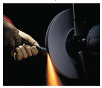
The 3M<sup>™</sup> XR Metalworking Wheel is loaded with mineral and is designed for demanding applications such as removing sharp burrs that may drastically reduce the life of a non-woven abrasive or rubber bonded wheel.
