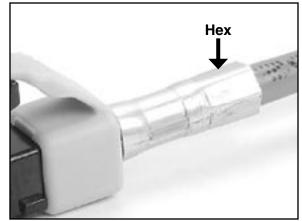
15.5 Slide boot over crimp until boot is flush against the connector.
