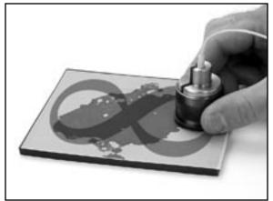
19.8 Leaving polishing jig assembly positioned on the lapping film rotate 180 degrees. Perform 4 additional figure eights.
