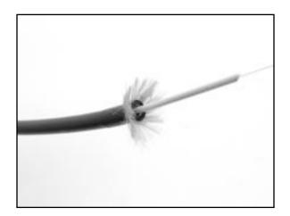
Using the 3M<sup>™</sup> Stripping Tool 6365-ST, remove the buffer in small increments until 21–22 mm (approx. 7/8") of buffer is left.
