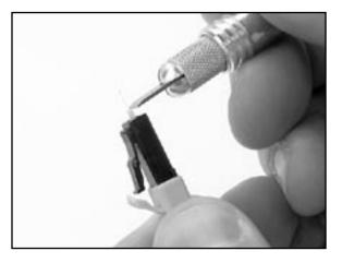
16.3 Pull the fiber straight away from the connector. Pull along the axis of the fiber, not to one side or the other. If the fiber does not pull away, score the fiber again.
