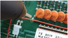
Product assembly with a slim profile to help operators apply adhesive more accurately.
