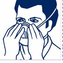
5. The seal of the respirator on the face should be fit-checked prior to wearing in the work area. a) Cover the front of the respirator with both hands, being careful not to disturb the position of respirator. b) Inhale sharply. A negative pressure should be felt inside the respirator. If any leakage is detected, adjust position of respirator and/or tension of strap. Retest the seal. Repeat the procedure until the respirator is sealed properly.
