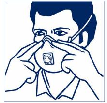
4. Place the fingertips of both hands at the top of the metal nosepiece. Mould the nosepiece to the shape of your nose by pushing inward while moving your fingertips down both sides of the nosepiece. Pinching the nosepiece using one hand may result in less effective respirator performance.
