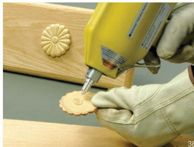
Bond wood or plastic trim to wood cabinet doors.
