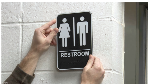
233 3M™ Double Coated Urethane Foam Tapes bond plastic signs to painted cinder block. The foam fills gaps between irregular surfaces. Various foam thicknesses are available for surface conformance based on the degree of roughness.
