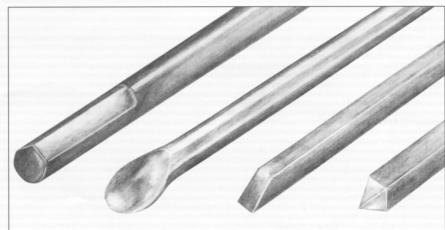
Knife Edge sharpened to break through oxides and conformal coatings Standard Clip "Duck Billed," will not "roll off" round or flat leads SOIC conforms to device lead PLCC mates with flat surface of "J" Lead
