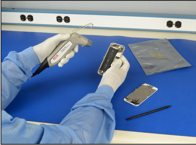
Figure 5. Using the Ionized Air Gun
