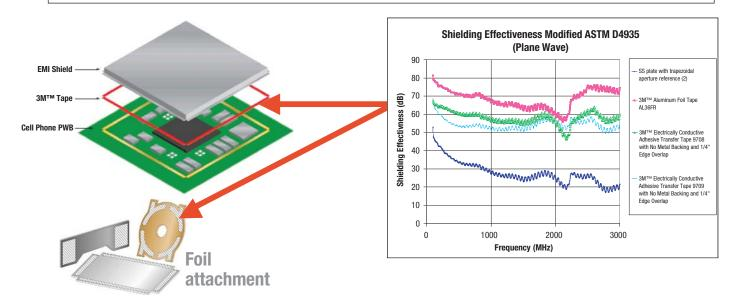
3M<sup>TM</sup> Electrically Conductive Adhesive Transfer Tapes 9703, 9705, 9706, 9709, 9709S, 9709SL, 9712, 9713, 9723, 7805 and 7810 can provide FPC grounding and tapes 9707, 9709, 9709S, 9709SL, 7805 and 7810 can increase the effective EMI Shielding through the bond line thickness leading to improved product EMI Shielding performance of the FPC.
