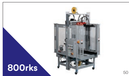
800rks 3M-Matic™ Case Sealer 800rks is a random king size case sealer that automatically adjusts for case height and width and is capable of sealing up to 10 cases per minute, using tape widths from 48mm to 72mm wide.
