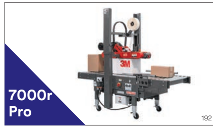
7000r Pro 3M-Matic™ Random Case Sealer 7000r Pro is a semi-automatic random case sealer that automatically adjusts for case height and width and is capable of sealing 24 cases per minute, using tape widths from 36mm to 48mm wide.
