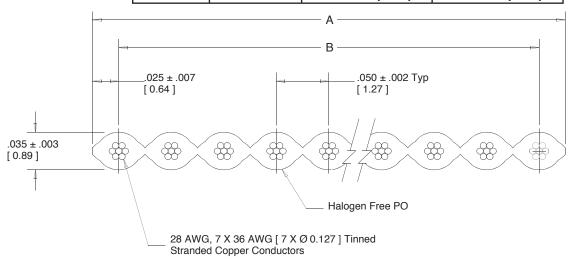
1. Blue marking on one edge of cable designates wire #1.
