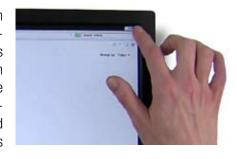
Corner and edge performance exceeds 99% accuracy, so whether drawing or activating a corner located button, the 3M PCT system will deliver the performance expected by the user.
