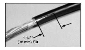
3.03 Make a 1" (25 mm) slit in the outer sheath and shield. Lift corners for base insertion.
