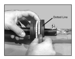
5.04 **End seal cutting is optional,** but makes closing of closure easier with larger diameter cable. If end seal is not cut, then compress SLiC end by using a knife to slit through thin plastic membrane.
