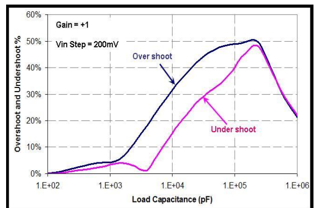
Small-Signal Over-Shoot % vs. C LOAD , Gain = +1
