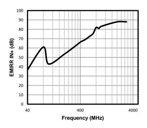
Figure 3. TP2311 EMIRR IN+ vs Frequency
