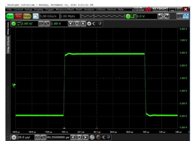
Voltage: 2V/div for Output, Time: 20us/div G=10, VREF = GND; VIN=1VPP, Load R=10K C=100pF Figure 24 Large-Signal Pulse Response
