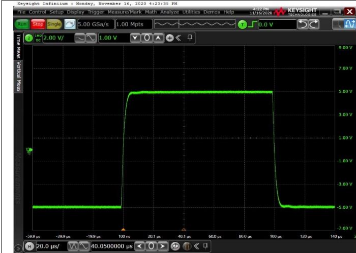
Voltage: 2V/div for Output, Time: 20us/div G=100, VREF = GND; VIN=0.1VPP, Load R=10K C=100pF Figure 25 Large-Signal Pulse Response
