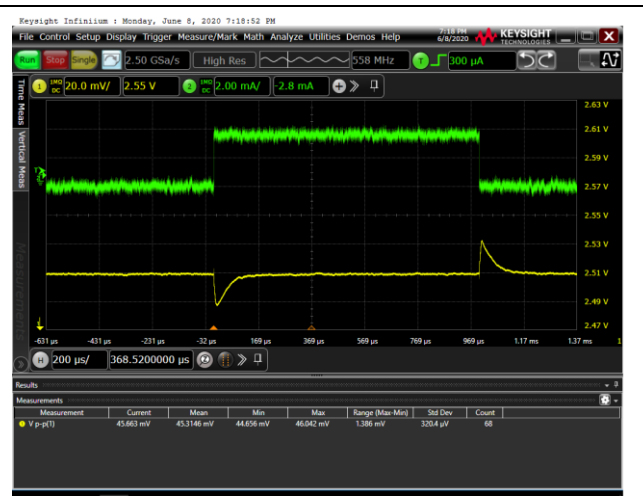
Figure 14. Load Transient, \pm 2\text{ mA} , V_{IN} = 2.8\text{ V} , C_{IN} = 1\ \mu\text{F} , C_{OUT} = 1\ \mu\text{F} , 20 mV/div
