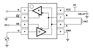
Figure 7. Loopback Test Circuit
