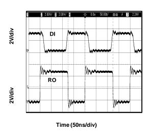
Figure 8. Loopback Test at 10Mbps/5V
