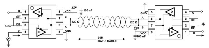
Figure 10. 10Mbps Data Rate With 30M CAT5 Cable Test Circuit
