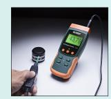
Extech's SDL900 measures and datalogs both AC and DC Magnetic Field in Gauss and mT (milli Tesla) with a uniaxial Hall effect sensor and built-in ATC. Internal memory stores up to 99 readings, while SD memory card (included) allows continuous datalogging and readings can easily be exported to an Excel<sup>®</sup> format for further analysis.
