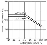
1-(2). Load current vs. ambient temperature characteristics
