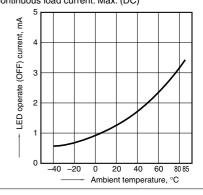
6. LED reverse (ON) current vs. ambient temperature characteristics Sample: All types;
