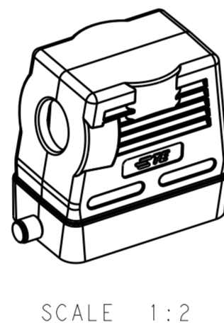
TYPE-3: H10B HOOD, HIGH CONSTRUCTION, SIDE ENTRY, 2 EAR 类型-3: H10B上壳, 高结构, 侧出, 2耳
