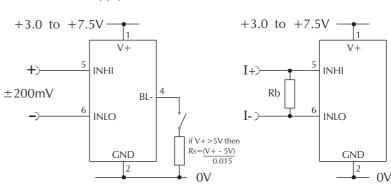
Measuring an input voltage referenced to a floating supply, i.e. the input voltage and the meter's power supply are isolated from each other. Ensure solder link LCOM is closed. Measuring a current from a circuit which is floating with respect to the DPM's supply, i.e. the current and the meter's power supply are isolated from each other. Ensure solder link LCOM is closed.
