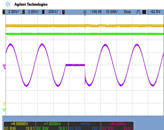
Figure 12 - AC drop out 12ms (10ms/div) CH1: V1 (2V/div) CH2: VSB (2V/div) CH3: Vin (200V/div)
