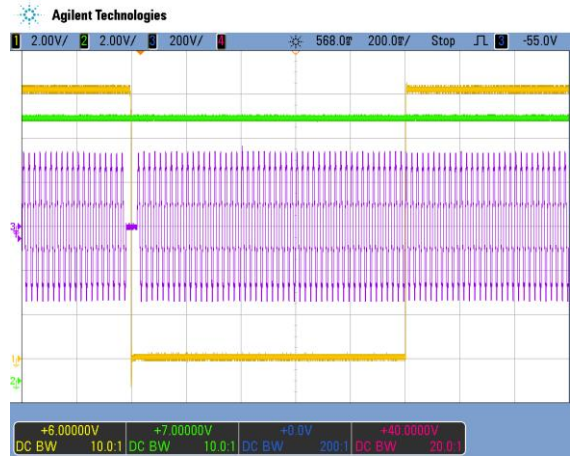
Figure 14 - AC drop out 40 ms, full load (200 ms/div), V1 restart after 1 sec CH1: V1 (5 V/div); CH2: VSB (2 V/div); CH3: I1 (200 V/div)
