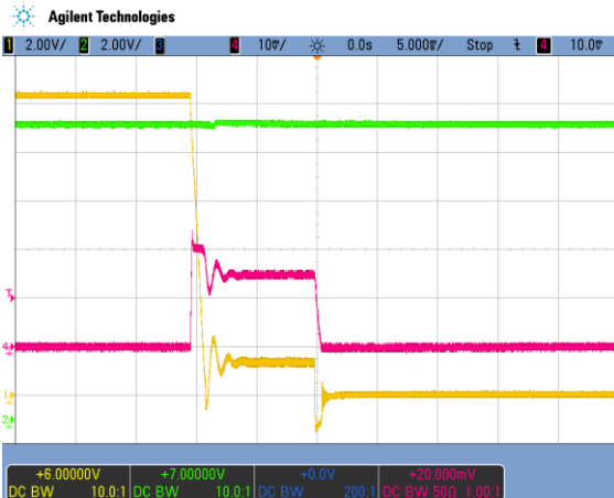
Figure 11 - Short circuit on V1 (50ms/div) CH1: V1 (2V/div) CH2: VSB (2V/div) CH4: I1 (200A/div)
