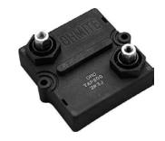
Ohmite's TAP800 Series dissipates 800 watts of power when used with a liquid or air cooled heat sink system. The Ohmite CP4 (http://www.ohmite. com/cat/sink\_cp4.pdf) is an example of properly designed heat sink. The TAP800 rounds out 600 watt (TAP600) and 1000 watt (TAP1000) product offerings. Applications include variable speed drives, power supplies, robotics, motor control, control devices, and other power designs.
