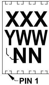
14-Lead SOIC (150 mil) (MCP6444)
