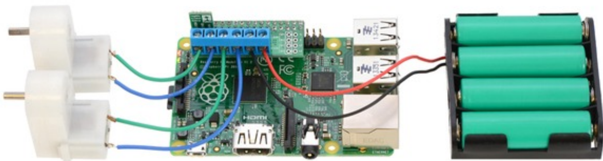
Driving motors with an assembled Pololu DRV8835 Dual Motor Driver Kit for Raspberry Pi B+. A step-up/step-down regulator provides 5 V to the Raspberry Pi.
