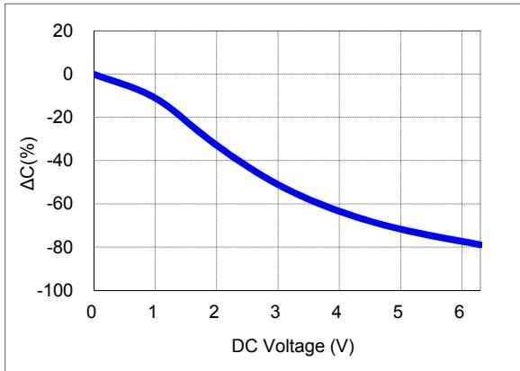
4) Bias TCC characteristics (Agilent 4284A, 1kHz, 1Vrms, 3.15Vdc)
