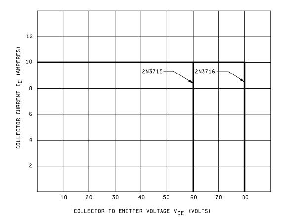
FIGURE 6. Safe operating area for switching between saturation and cutoff (clamped inductive load).
