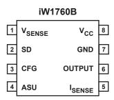
Figure 4.1: 8 Lead SOIC-8 Package
