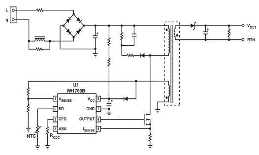
Figure 3.2 : iW1760B Typical Application Circuit (Alternative Circuit without Using Active Start-up Device)
