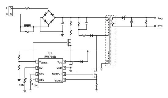
Figure 3.1 : iW1760B Typical Application Circuit
