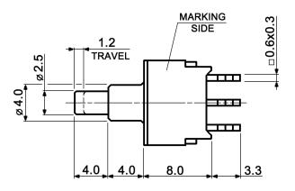
When looking at the marking side, the normally closed contacts are on the right hand side.
