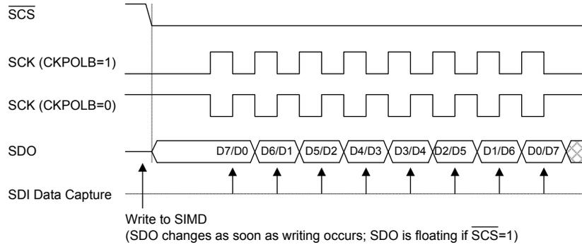
Note: For SPI slave mode, if SIMEN=1 and CSEN=0, SPI is always enabled and ignores the SCS level.
