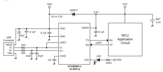
Note: 1. The  $V_{\text{CC}}$  voltage must be less than the  $V_{\text{DD}}$  voltage. The  $V_{\text{CC}}$  supply can be sourced from a Li-battery.
