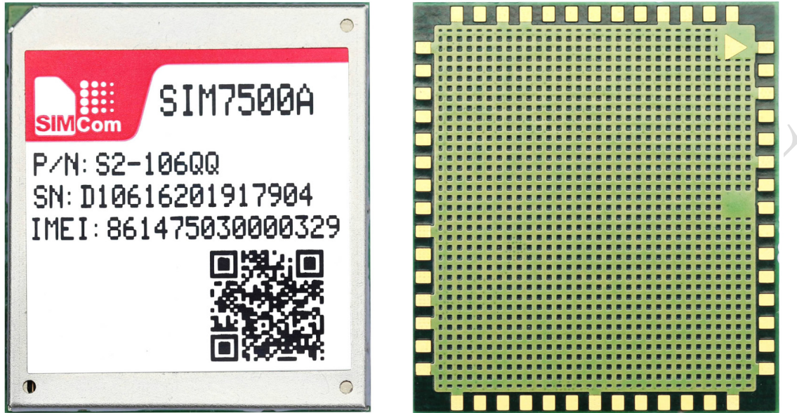
Figure 33: Top and bottom view of Module
