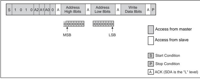
Note: In the MB85RC256V, input "0" to the most significant bit of the higher address byte because the address is expressed with 15 bits.
