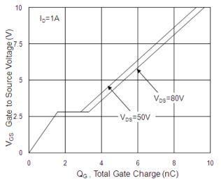
Fig.4 Gate-Charge Characteristics
