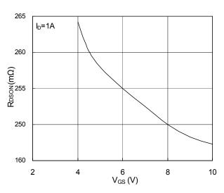
Fig.2 On-Resistance vs. Gate-Source
