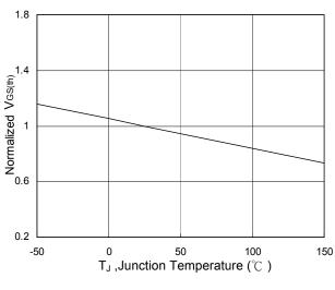
Fig.5 Normalized  $V_{GS(th)}$  vs. T<sub>J</sub>
