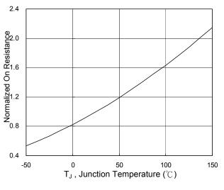
Fig.6 Normalized  $R_{\text{DSON}}$  vs.  $T_{\text{J}}$
