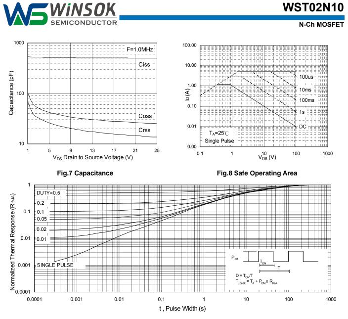
Fig.9 Normalized Maximum Transient Thermal Impedance
